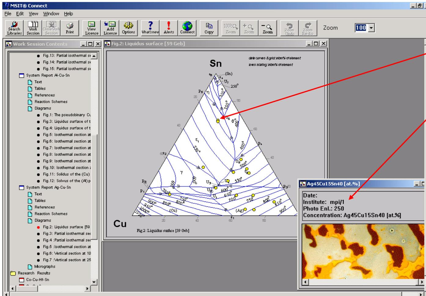
The screenshot displays the MSI@ Connect software interface. The main window shows a ternary phase diagram for the Ag-Cu-Sn system, titled "Fig.2: Liquidus surface [59 Geb]". The diagram plots temperature against the composition of Ag, Cu, and Sn. A red dot is placed on the liquidus surface at approximately 250°C and 40% Ag. A red arrow points from this dot to a pop-up window titled "Ag45Cu15Sn40 [at.%]". This window contains the following information:
